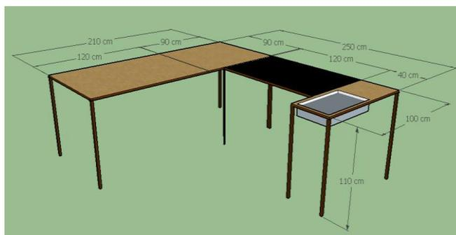
**Figure 5. Schematic Diagram of the Ergonomic Workstation**
