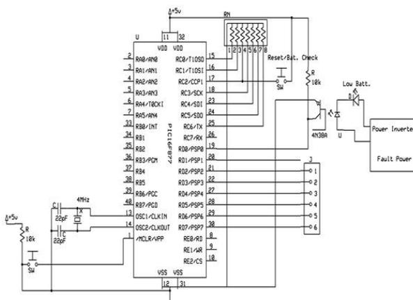
Figure 1. Microcontroller Unit Core
