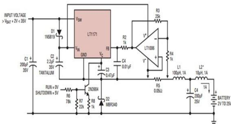
**Figure 3. Schematic Diagram of Buck-Boost**
