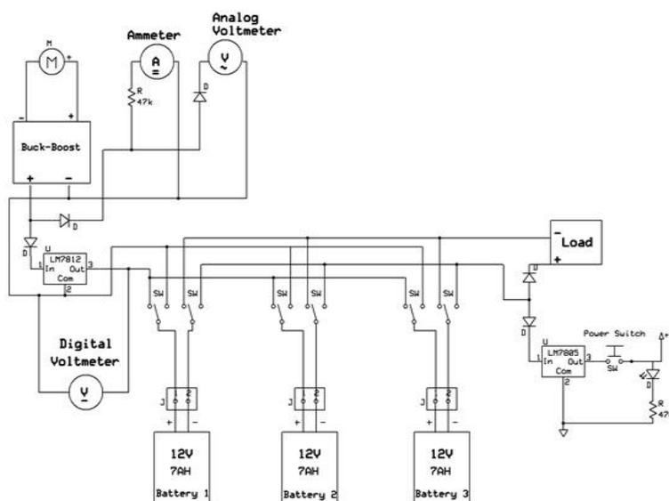
Figure 2. Schematic Diagram of the Batteries
