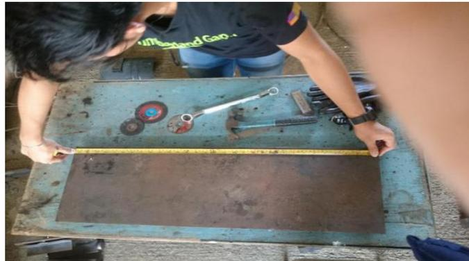
2. Laying out of the design and sizes directly to materials using scribe and steel rule
