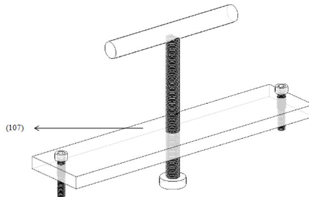
**Figure 8. Schematic view of the structure of the Clamping Plate and Screw**
