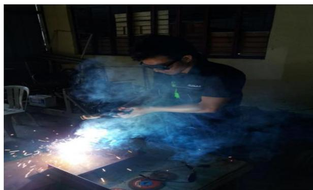
8. Welding the sub-assembly of clamp support guide using arc welding machine
