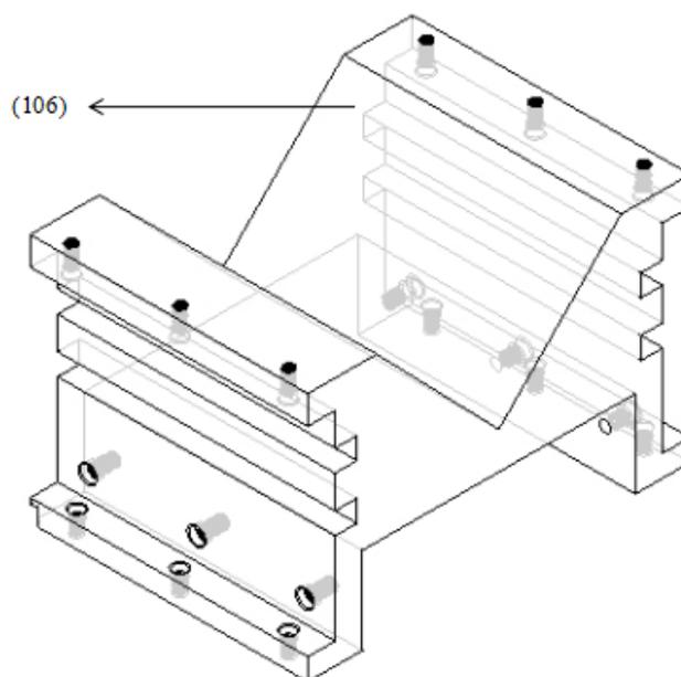
**Figure 7. Schematic View of the Structure of the Reversible V-Block**
