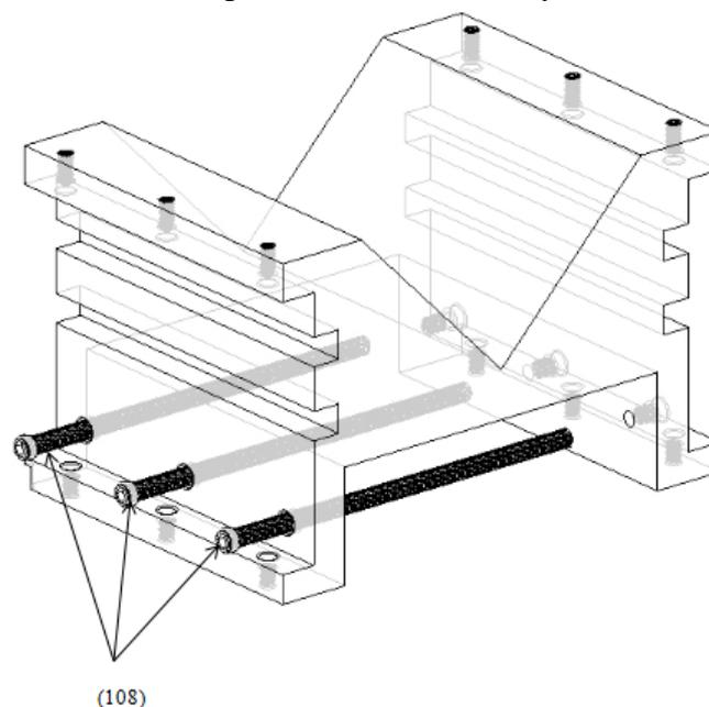
**Figure 9. Schematic View of the Structure of the Clamping Bolts**
