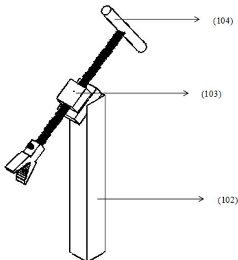
**Figure 4. Schematic view of the Structure of the Clamping support Assembly and Clamping Support Guide**
