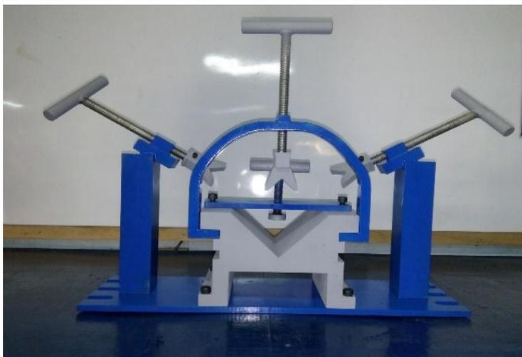
**Figure 10. The Completed Assembly of Multi-Functional Clamping Device**
