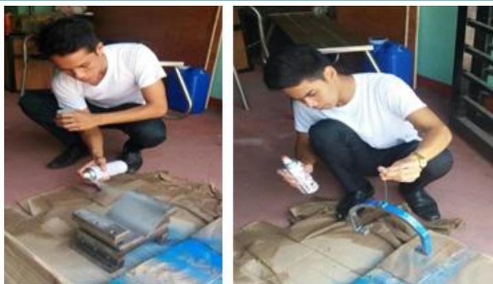
9. Coating the sub-assembly using spray paint
