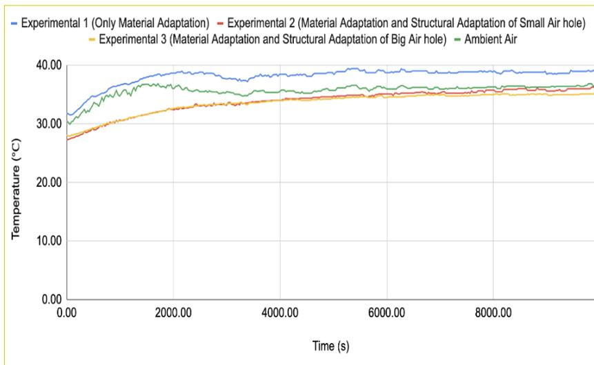
**Figure 7.** Time-series plot of heat index in structures with and without structural adaptations throughout the experimental period. The plot shows heat index for each structure across different phases of the experiment. The plot also illustrates the heat index as a reference point.
