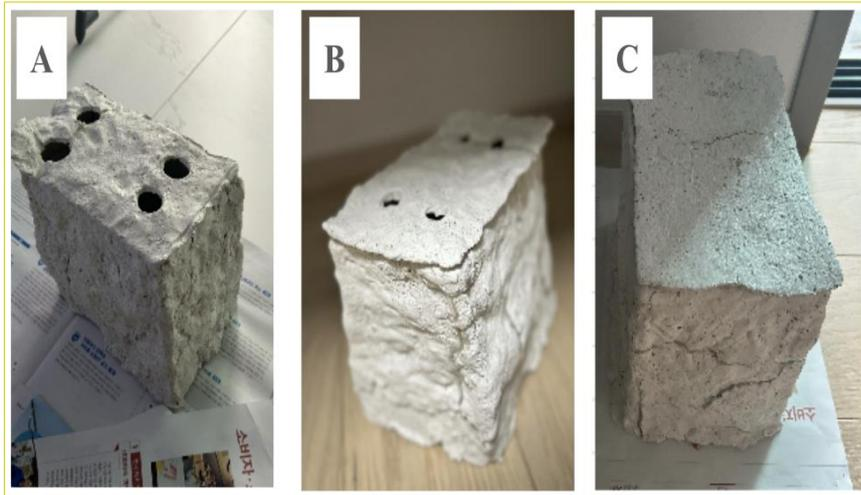
**Figure 2.** Created structures inspired by termite mound features. (A) Both structurally and materially modified with a large-radius air hole. (B) Both structurally and materially modified with a small radius air hole. (C) Only materially modified without any air holes.
