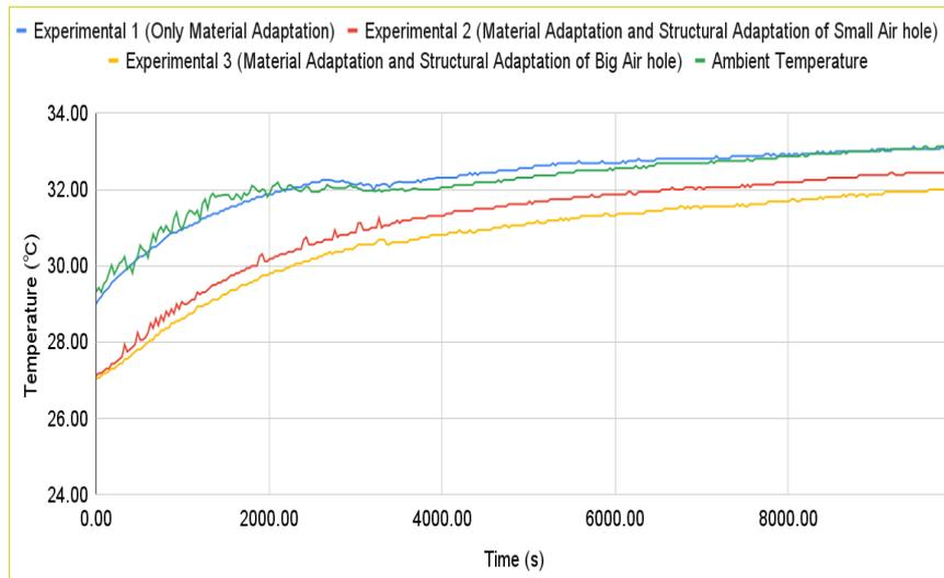
**Figure 3.** Time-series plot of internal temperature in structures with and without structural adaptations. The plot shows the thermal performance of each structure across different phases of the experiment. The plot also illustrates the ambient air temperature to provide a benchmark for the interior temperatures.
