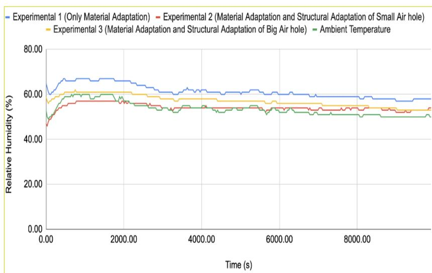
**Figure 5.** Time-series plot of relative humidity in structures with and without structural adaptations throughout the experimental period. The plot shows relative humidity for each structure across different phases of the experiment. The plot also illustrates the ambient air relative humidity level to provide a benchmark for the interior relative humidity.
