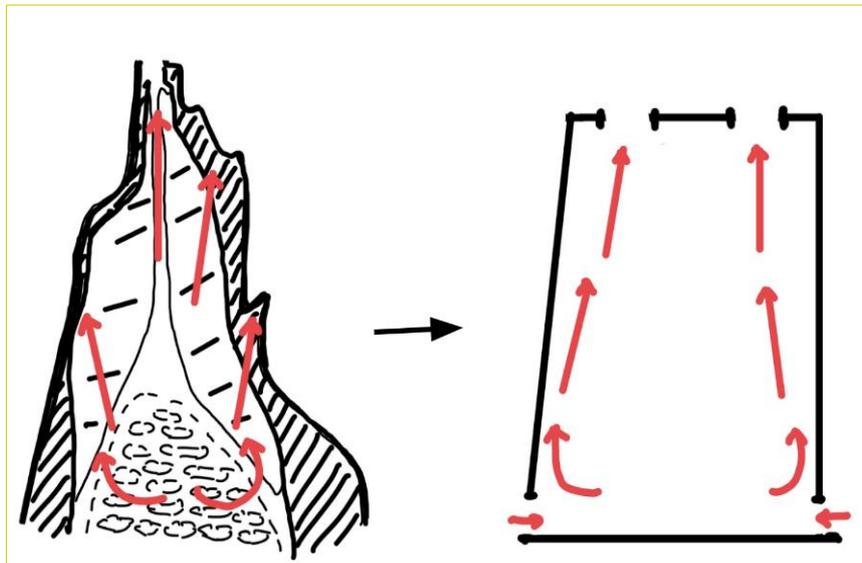
**Figure 1.** Natural ventilation in termite mounds (left) and its adaptation in this study (right). Both illustrations mark the air circulation path by red arrows. The illustration on the left demonstrates the air circulation path in a real-life termite mound (adapted from Jost [9]). The illustration on the right demonstrates the air circulation path in a simplified termite mound design.
