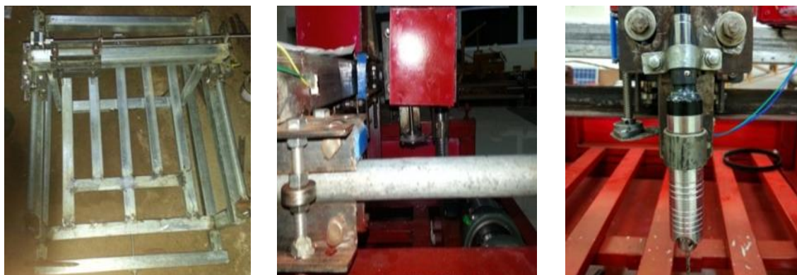
Figure 2. Mechanical Assembly for X axis, Y axis and Z axis
