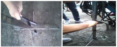
5. Clean the welded portion of the boom and the sensor holder. This is to done to ensure a tight and mounting angle for a better stand of the device
