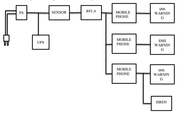
Figure 4. Block Diagram of Water Level Sensing and Warning Device with Short Message Service (SMS) Notification
