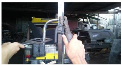
3. Weld the sensor holder on the side of the boom. Holder must be bent downside and the sensor face must be in a downward position
